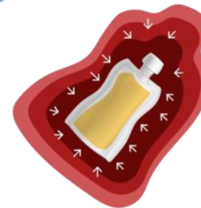
STERILIZATION TEMPERATURE (121 °C / 250 °F) IS ACHIEVED AS PRESSURE REACHES 6000 BAR / 87,000 PSI DUE TO ADIABATIC COMPRESSION HEATING PROCESSING TIME IS DRASTICALLY REDUCED
