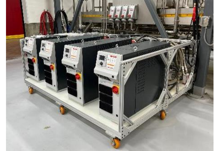
TCU- CLOSED LOOP COOLING UNITS
